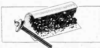
Pertrix battery cell showing the grooved carbon and saccus depolariser.
