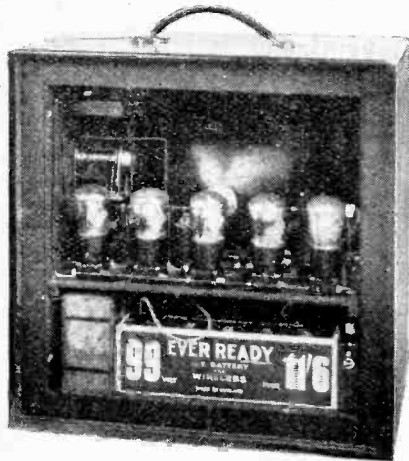
The Pegasus portable receiver with back cover removed.
