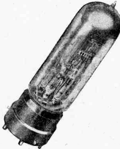
Loewe multiple valve (triple) containing detector with contact for reaction and two resistance-coupled L.F. stages.
